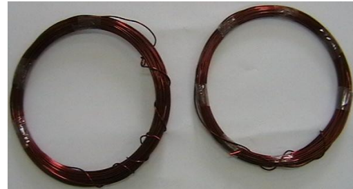
Fig. 13. Two ring-shaped armature windings.
