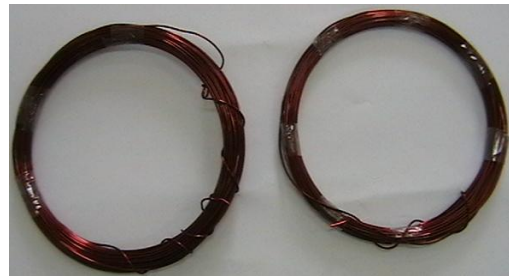
Fig. 13. Two ring-shaped armature windings.
