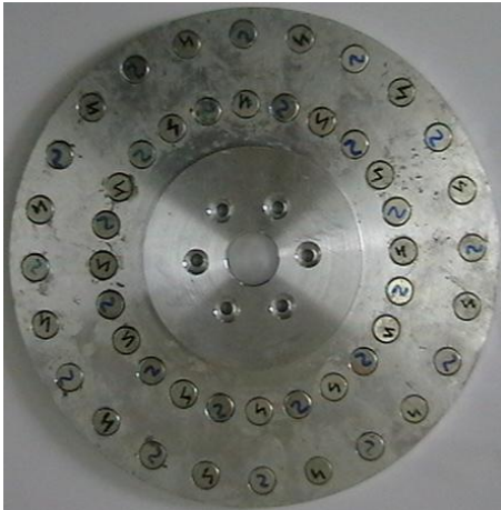
Fig. 11. Rotor Disk with circular flat shaped PMs.
