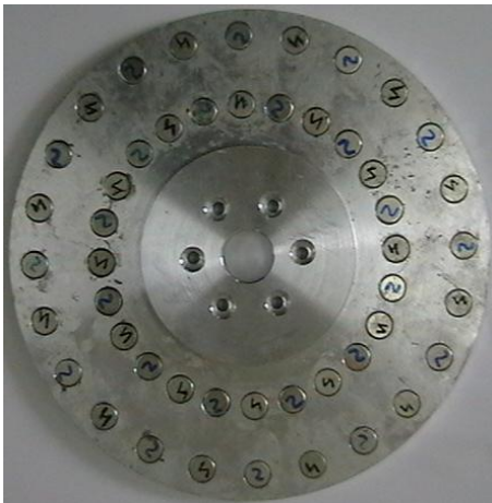
Fig. 11. Rotor Disk with circular flat shaped PMs.
